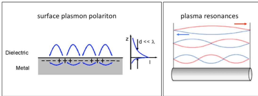
*Fig.1 **Left:** pictorial representation of a Surface Plasmon Polariton (SPP). The blue lines indicate the electromagnetic field sustained by the charge distribution accumulated at the surface. In the small graph, the spatial confinement of such an SPP field is highlighted. **Right:** when traveling SPPs reflect from the edges of a nanostructure, such as a nanowire, a standing-wave can be created; this is referred to as a plasma resonance*
