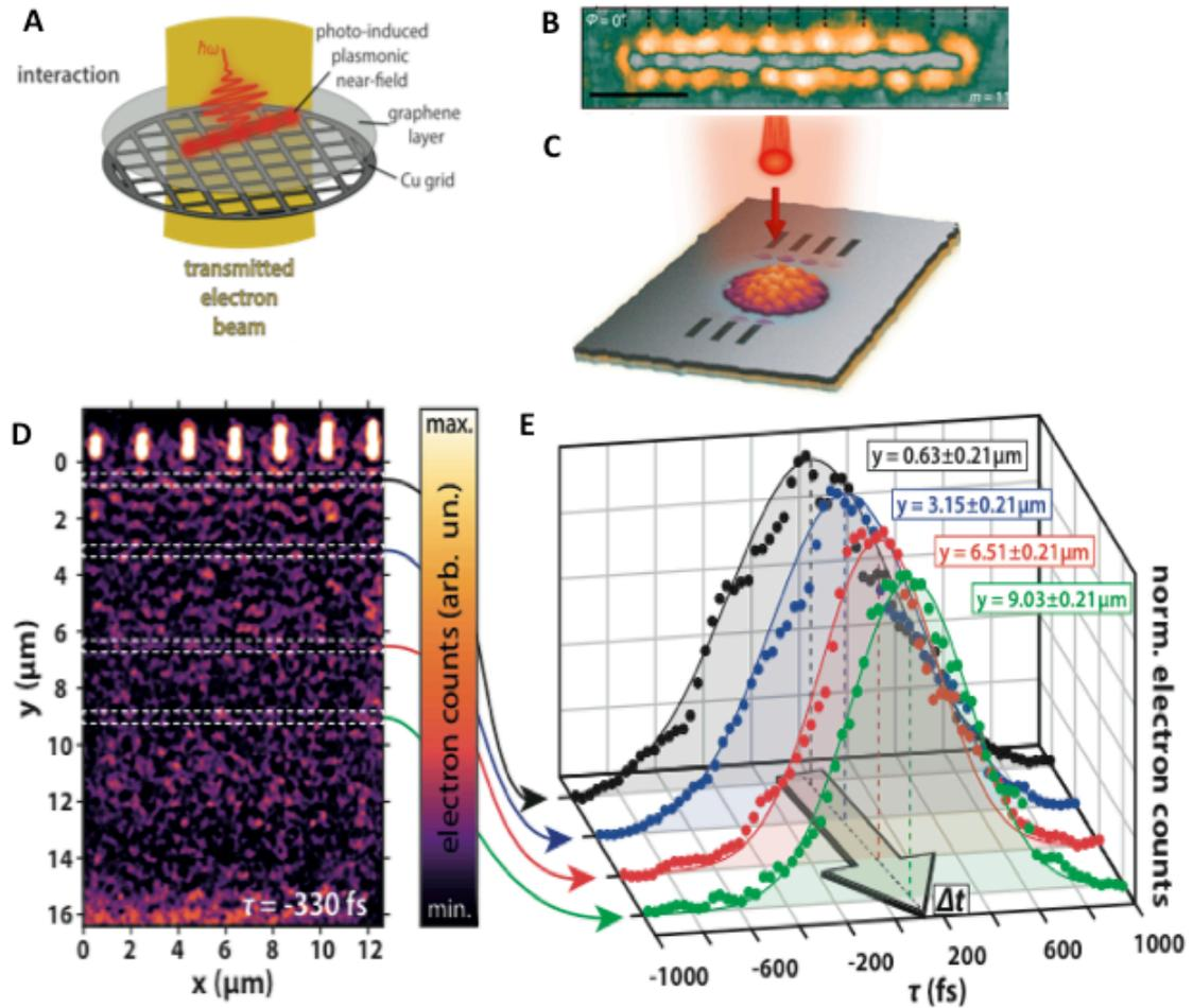
*Fig. 3 A: Schematics of the photoexcitation of SPPs on a nanostructure. B: ultrafast TEM image of a plasma resonance on a single nanowire. C: ultrafast TEM image of the plasmon-plasmon interference generated by an array of nano-antennas. D: single frame of a movie capturing the propagation of SPPs in a thin film once they are radiated by the antenna array at the top of the image. E: Temporal evolution of the SPP propagation*
