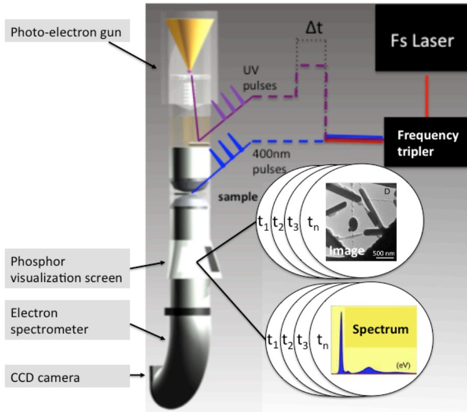
*Fig. 2: Schematics of an ultrafast TEM, see text.*
